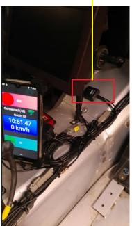
GPS antenna to be installed on the roof (or back window inside).
