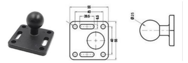
The device will be attached to a 1 inch ball head as shown in the picture above. This ball mount must be attached to the vehicle with tight screws at a location as described above. The diameter of the screw holes is 6.5mm and the distance between the holes is 40mm. When mounting on the dashboard, a support plate must be attached to the back to prevent the screws from breaking through the plate in the event of an accident to prevent the holder from flying around freely in the vehicle.
